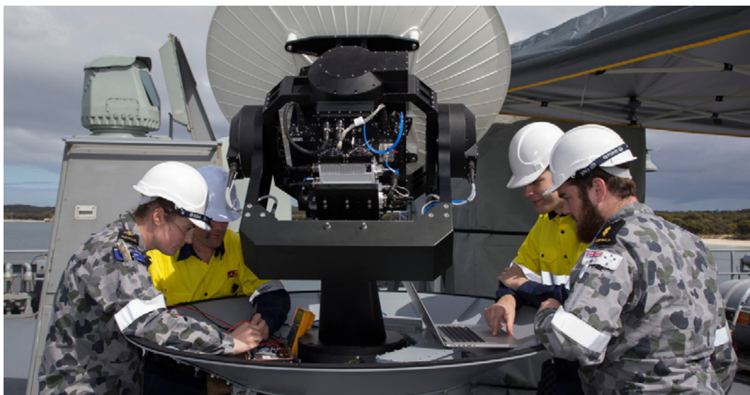
Sailors assist contractors from EM Solutions during a trial of the Tri-Band SATCOM terminal during the installation of a new Wi-Fi network.
