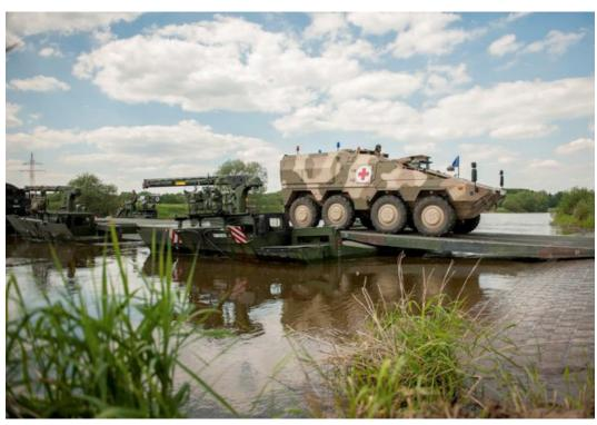
A German Boxer crossing a temporary bridge formed by several UK and German M3 Amphibious Rigs during a joint UK/ German bridging operation
