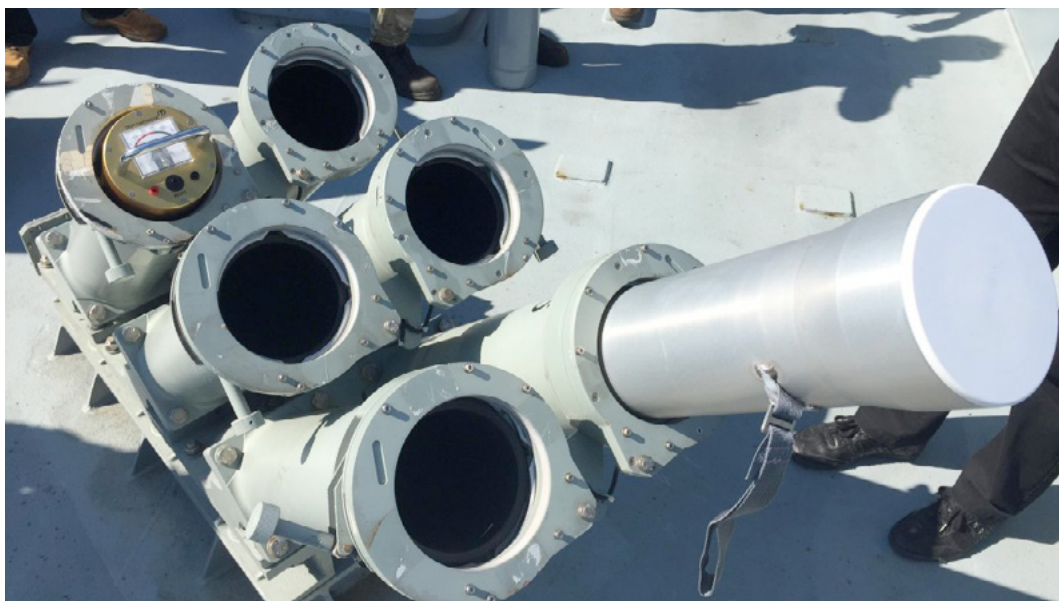
Terma's C-Guard Decoy Launching System with a CANTO Anti-Torpedo Decoy and a Chemring Launch Module – together designated NATO standard CANTO 130mm.
