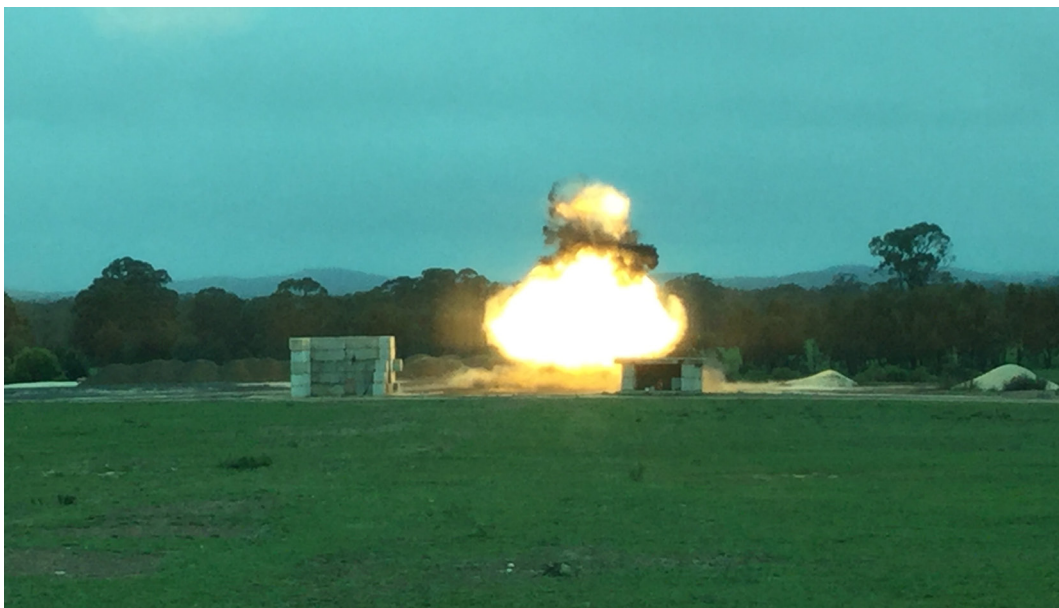
The test specimen was repeatedly blown up until the “bulge” in the steel produced a thinning of the hull.
