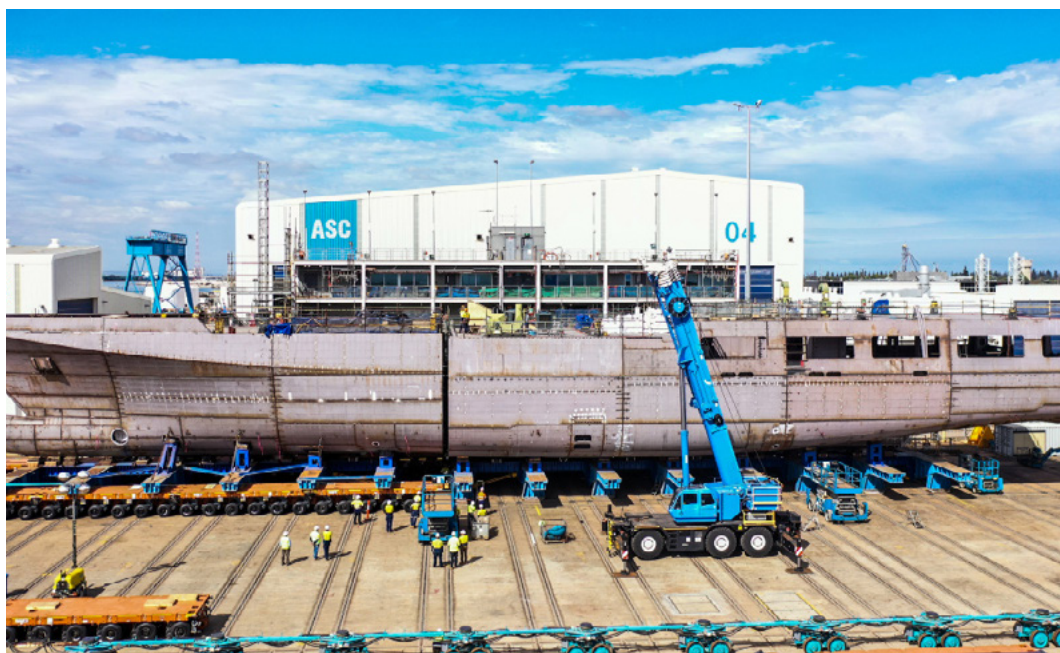
The two halves of the first OPV are brought together and welded to form a complete hull.
