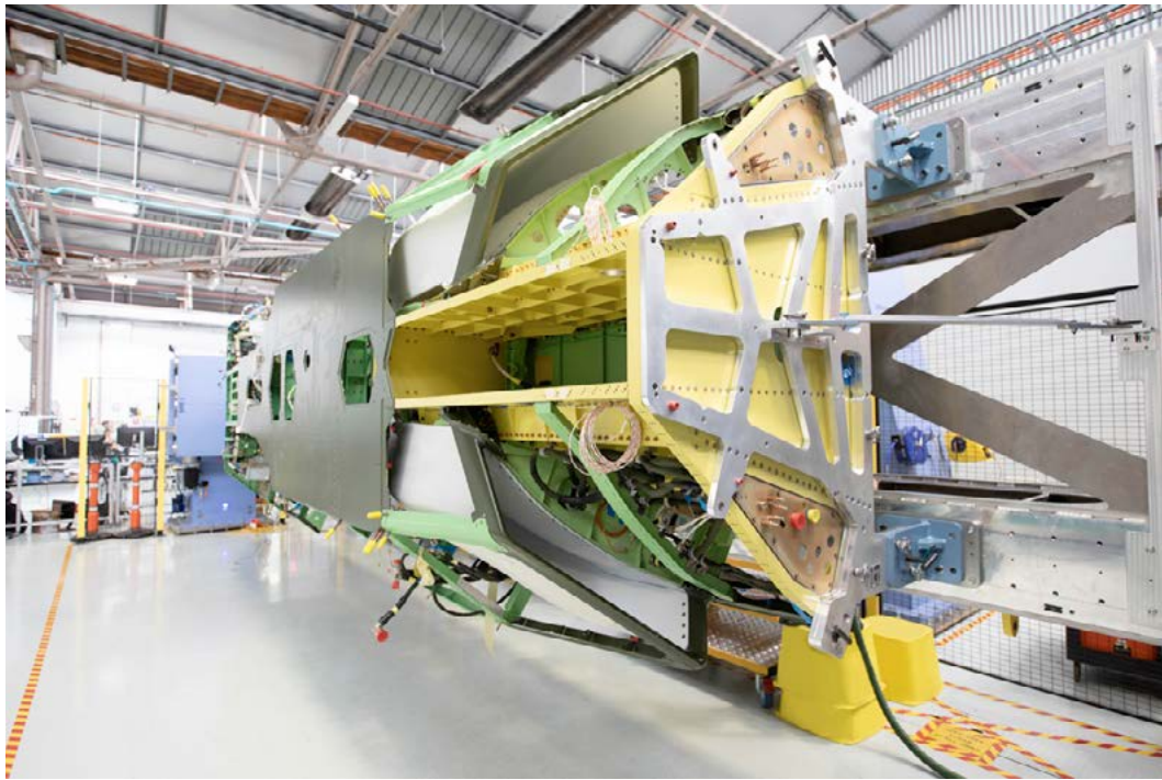
Boeing Australia has completed the major fuselage structural assembly for its first Loyal Wingman aircraft.
