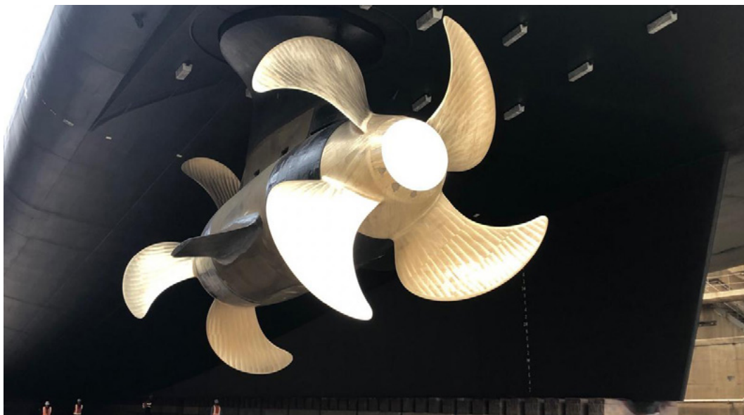
The completed pod installation includes a new four-blade propeller arrangement.
