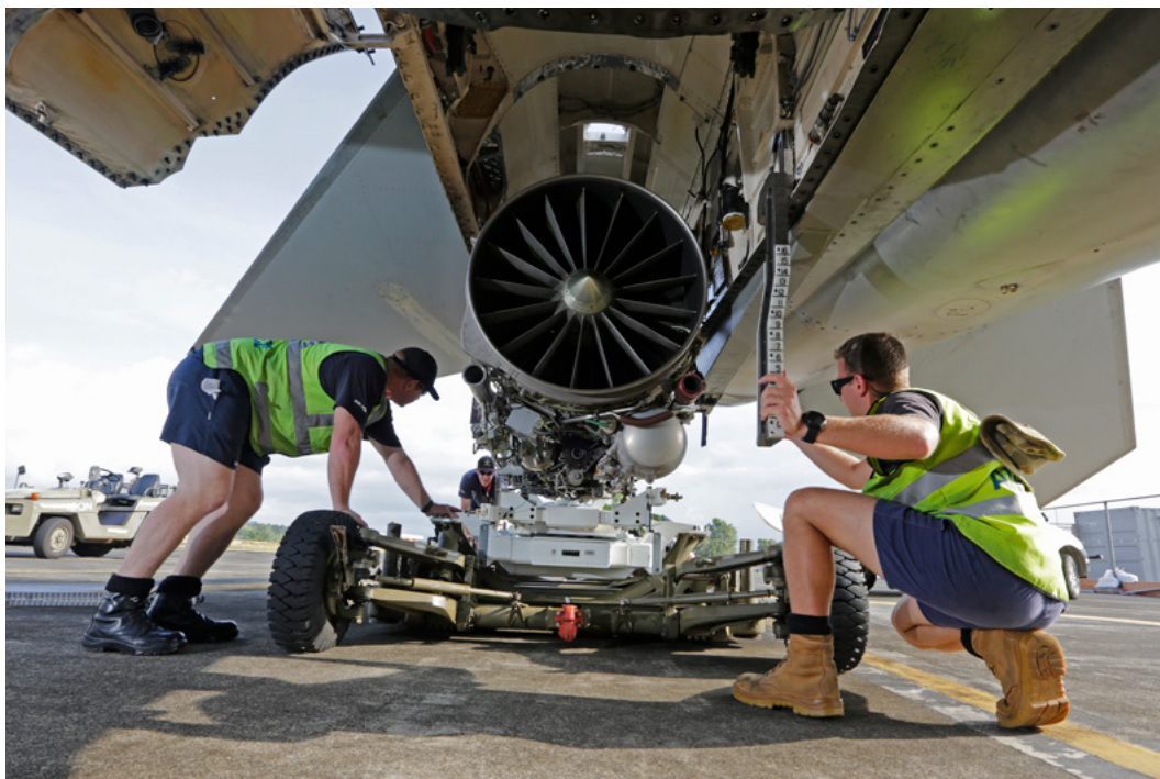
Aircraft Technicians from RAAF's No. 1 Squadron guide an F414 engine into position for an engine swap on a F/A-18F Super Hornet. DEFENCE
