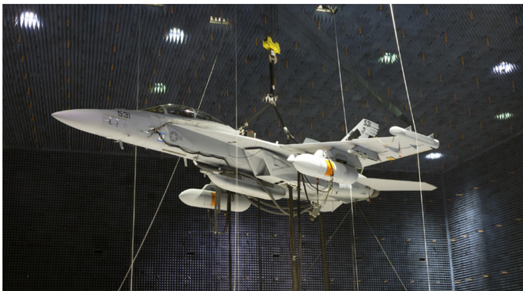
Two Next Generation Jammer Mid-Band pods, attached to an EA-18G Growler, undergo testing in the anechoic chamber. US NAVY
