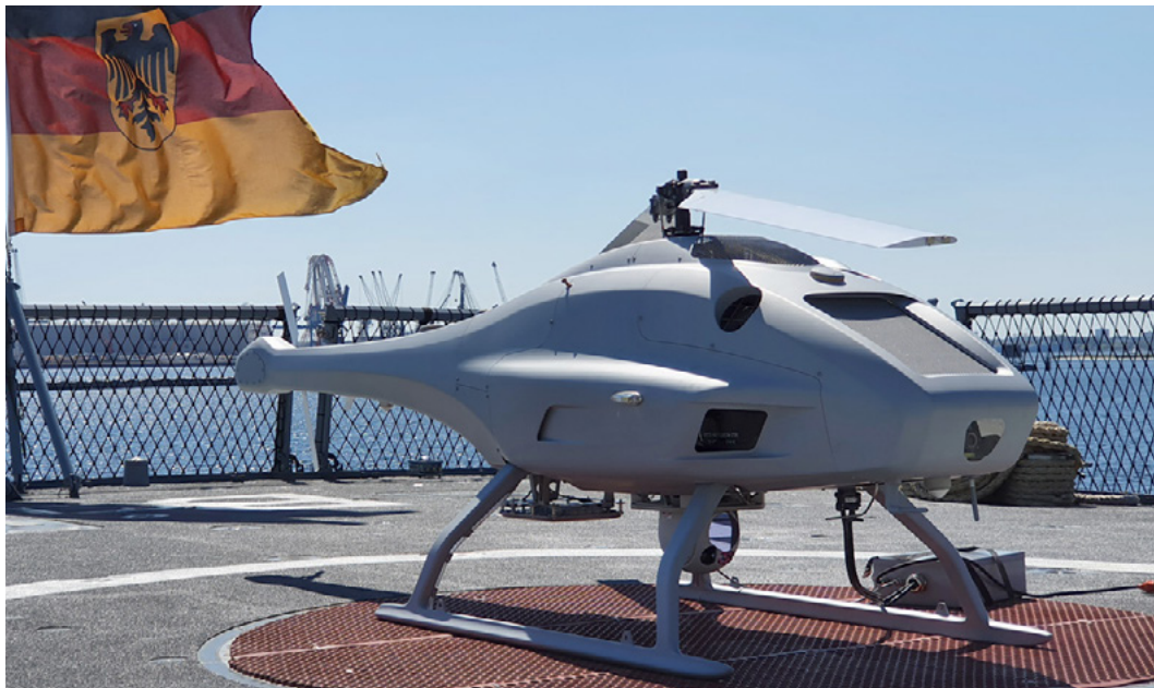
UMS' Skeldar V200 is the first UAV to autonomously take-off and land from a moving ship on operations.
