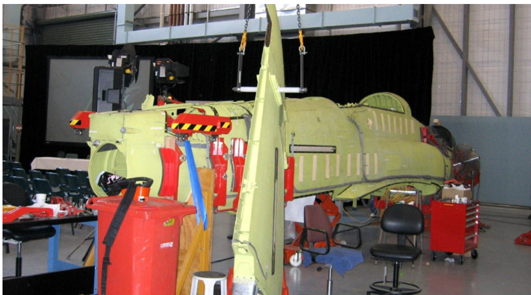
The Full-Scale Fatigue Test program began in February 2006.
