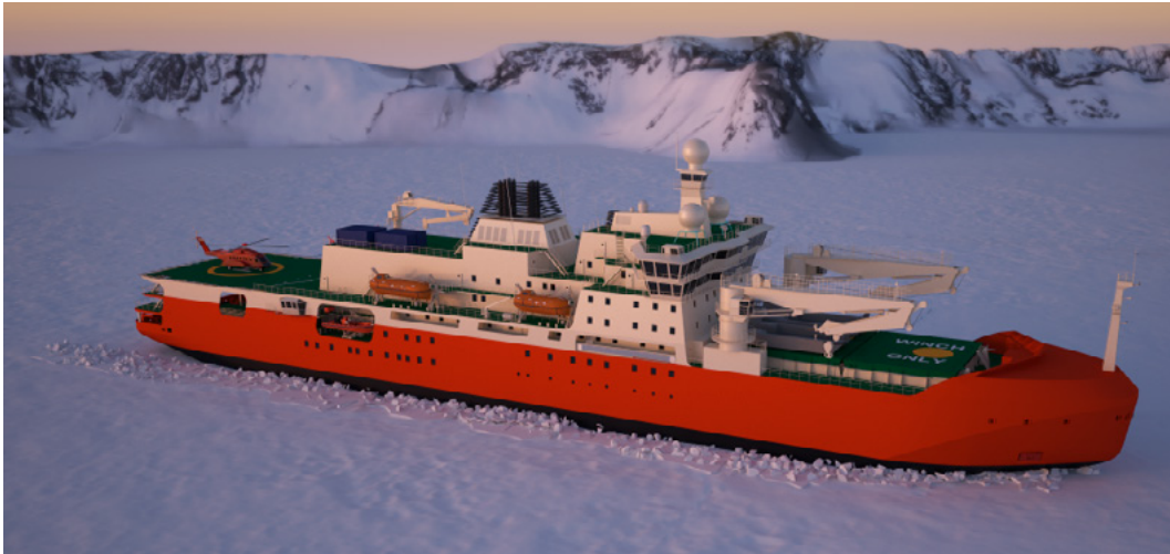
The RSV Nuyina will be able to break two-metre thick ice at a continuous speed of three knots. DAMEN/DMS MARITIME/KNUD E HANSEN
