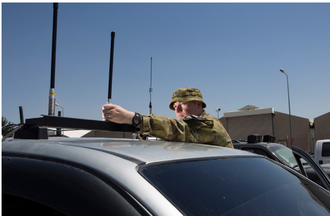
Major Geoffrey Small installs a silver shield electronic countermeasure device on a vehicle in Kabul, Afghanistan.
