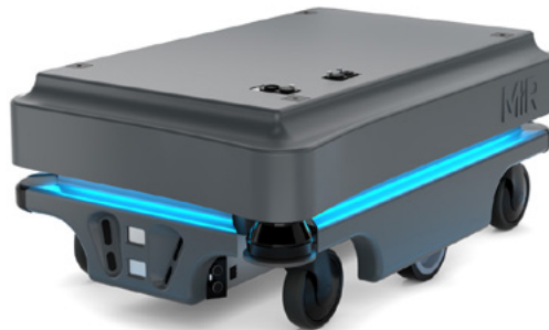
The Mir200 can carry up to 150 kg at a time. KONICA MINOLTA
