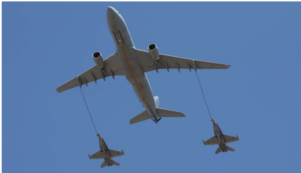
The problem hoses installed in Cobham's 905E refuelling pods installed under each wing of the RAAF's KC-30As. NIGEL PITTAWAY
